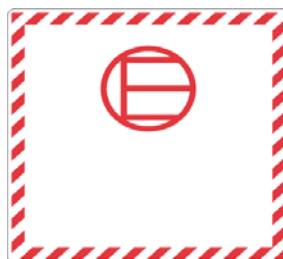
Figure 5. DOT –E, exempt quantity label, will also contain 4 digit number and material name
