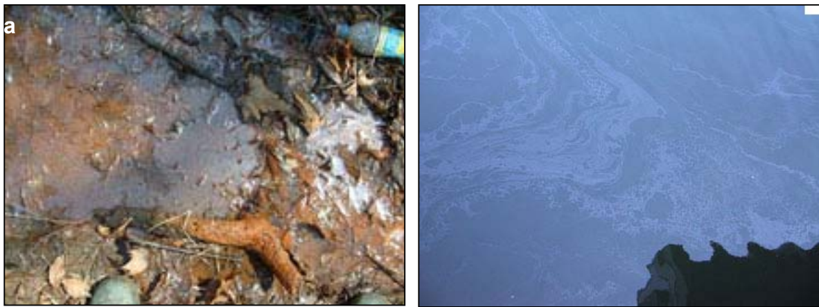
Synthetic versus Natural Sheen (a) Sheen from bacteria such as iron floc forms a sheet-like film that cracks if disturbed (b) Synthetic oil forms a swirling pattern suds
